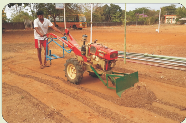
UAHS Designed power tiller operated Dozer has been accepted for farm trial in the year 2016
