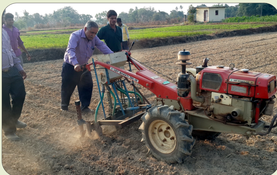
UAHS designed Power Tiller operated groundnut Seed drill is best suited for sowing groundnut seeds especially for small and marginal farmers
